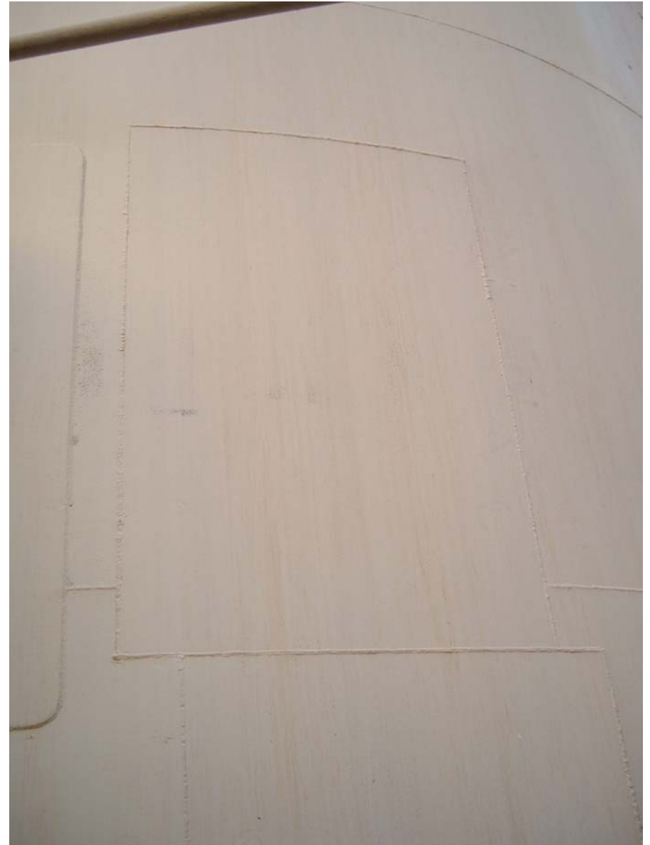
Fig. 10 – Typical shell insert plate with non-rounded corners
